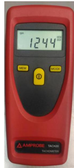
Figure 80. Maximum rpm reached in electric axial flux motor test.
